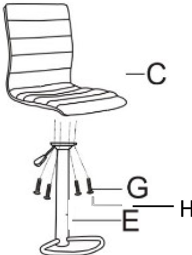
Attach Seat Base (E) to Seat (C) with Bolts (G) using Allen Key (H)
