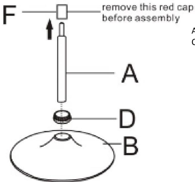
Attach Gaslift (A) and Star Base Cover (D) to Base (B)
